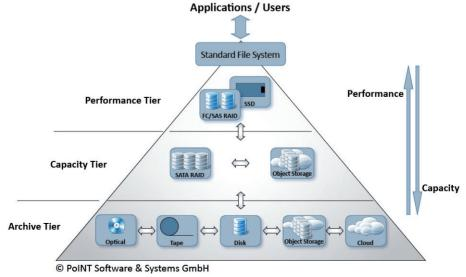
PoINT Storage Manager implements a tiered storage architecture homogeneously in an existing infrastructure. The "Single Path Access" concept assures that access to data via existing primary storage remains, thus no changes of existing applications are necessary.
