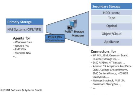
The integration of primary storage is implemented by "Agents", whereas secondary storage is utilized by "Connectors". In addition PoINT Storage Manager provides a CIFS interface through PoINT VFS (see section "CIFS Access by PoINT VFS").
