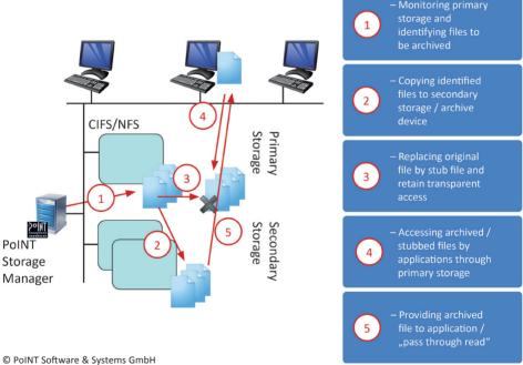
By this mechanism PoINT Storage Manager carries out a policy-based migration of files into the Capacity Tier and/or Archive Tier. The view of the primary storage file system does not change for users and applications, including access authorization (e.g. ACLs) and metadata. Access to migrated files is redirected automatically by the corresponding primary storage system to PoINT Storage Manager to supply the requested data from secondary storage.
