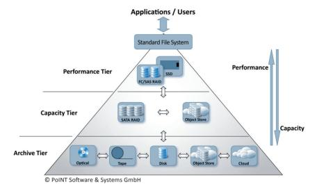
The topmost layer, the Performance Tier, is typically designed as primary storage and consists of high performance / highly available hard disk (e.g. FC/SAS RAID) combined with Flash/SSD. It is usually very expensive.
