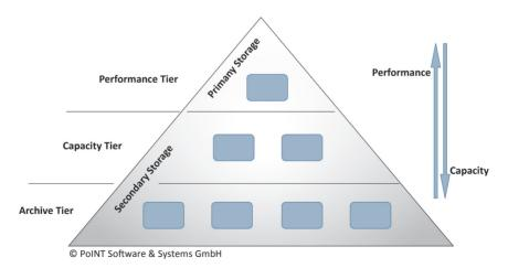
A predefined functionality is attributed to each tier: The Performance Tier consists of high performance storage; the Capacity Tier offers high capacity always accessible; the Archive Tier is intended for long-term preservation offering additional features with respect to compliant archiving.
